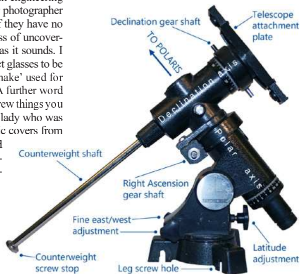
Right: Basic German equatorial mount, adjusted to the right angle for London. David Arditti.
