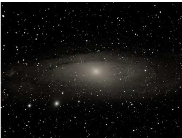
An image of M31 provided by Ron Morley, where stars show different distortions in different corners. This was found to be due to use of a damaged diagonal prism unit in the imaging train.
