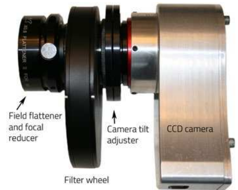
An imaging train for monochrome imaging with a short-focus refractor, incorporating a field flattener and tilt adjuster. All the components are threaded together, for rigidity. David Arditti
