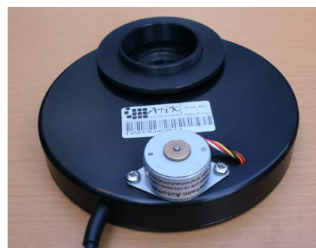
Atik motorised filter wheel for easily swapping 1.25-inch filters in the light path.
