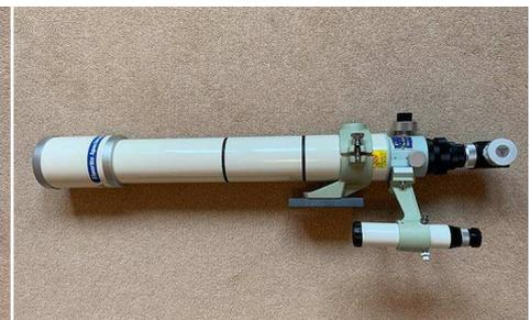
I have another telescope which is similarly convertible. The Takahashi FOA-60Q can be operated as a 60mm refractor in  $f/15$  mode or, by removing a section of the tube containing additional lenses, at  $f/8.8$ . Converting between configurations is relatively straightforward so long as one takes care to not cross-thread the fine threads on the tube components. Takahashi
