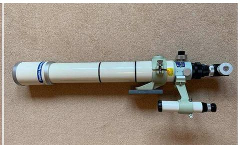
The FC-76 DCU. Top: the optical tube assembly in  $f/7.5$  configuration, with the Extender CQ 1.7x unit alongside. Bottom: the telescope in  $f/12.8$  configuration, with the Extender in place.
