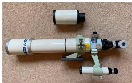
The FC-76 DCU. *Top*: the optical tube assembly in  $f/7.5$  configuration, with the Extender CQ 1.7x unit alongside. *Bottom*: the telescope in  $f/12.8$  configuration, with the Extender in place.
