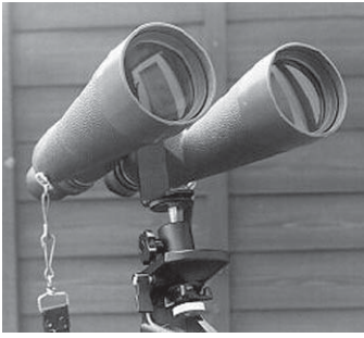
Figure 4. 16×70 Swift fixed to tripod head with angle bracket screwed to end of prism housing.
