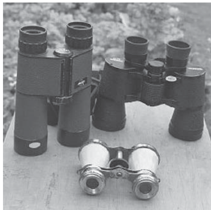
Figure 1. Three low power binoculars. Left to right: 8×40 Swift Trilyte (roof prisms), 3×20 opera glass, 8×42 Opticron (porro prisms).
