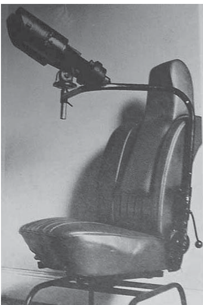
Figure 6. Modified car seat with steel bracket for binocular housing (courtesy The Astronomer , John Hosty, Peter Madej).
