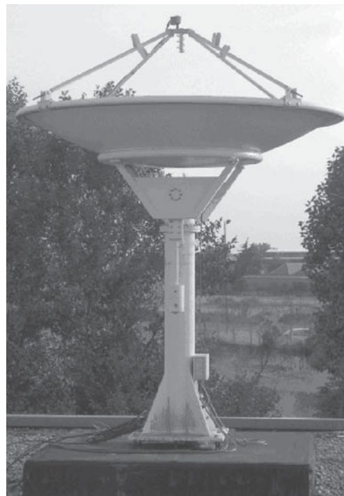
The 2.4m diameter, fully-steerable satellite antenna dish.
