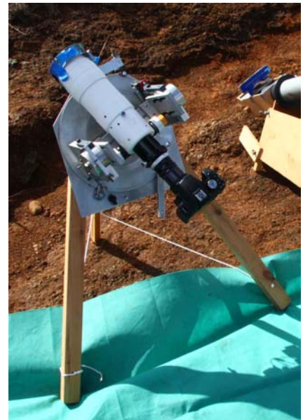
Figure 5. Megrez apochromatic refractor with 500D camera used for the HD video of the diamond rings.
