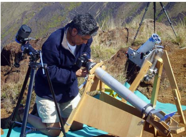
Figure 2. The author adjusting the 450D camera on the polar heliostat. The tripod on the left has the 600mm mirror lens. Next to the heliostat is the equatorial mount with the Megrez 72mm refractor. The tripod in the background has the 500D camera pointing at the landscape (picture by Martine Langridge).
