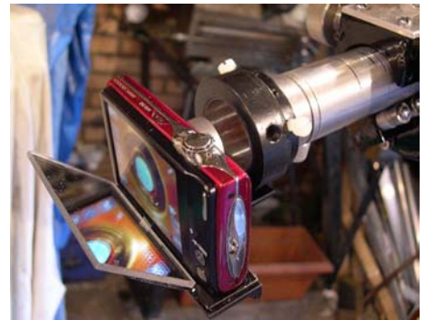
The Nikon 'Coolpix' compact camera mounted at the afocal position.
