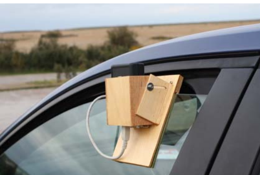
Figure 2. The simple clip-on window mounting for the SQM. The lead plugs into a laptop computer on the passenger seat.
