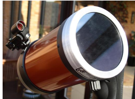
Figure 6: A solar filter fitted over the front of a Schmidt-Cassegrain telescope.
