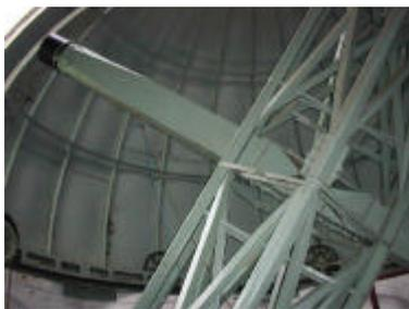
*The Northumberland equatorial as it is today. The dome was replaced in the 1930s, and the telescope had a new lens in 1988 to mark its 150<sup>th</sup> anniversary. Much of the rest of the telescope is unchanged since Professor Challis observed with it. For more details see <http://www.ast.cam.ac.uk/loA/northumberland.html>*
