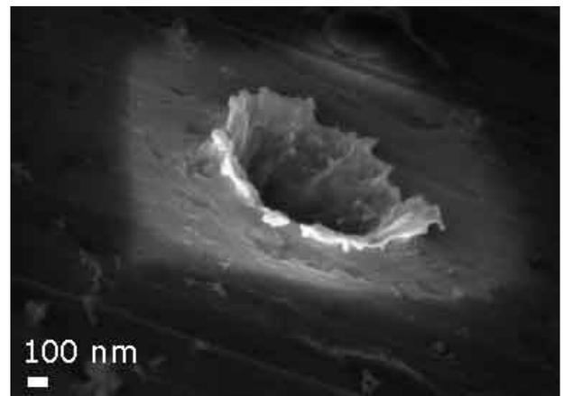
*Impact crater formed at 6 kms<sup>-1</sup> on aluminium foil strips of the Stardust collector tray. This image was taken with a scanning electron microscope OU/UL.*
