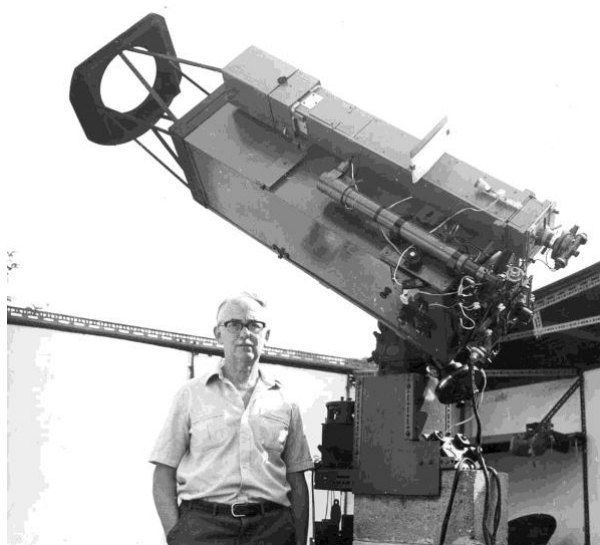
Mike Hendrie with his 25cm reflector. Note the micrometer on the guidescope
