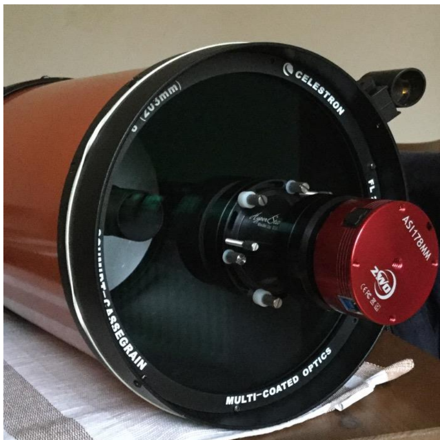
The C8 Hyperstar. A small mono planetary camera is attached. A 2in Baader UV/IR cut filter is mounted inside the Hyperstar (not visible)
