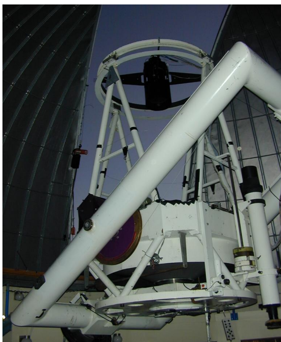
1.5-metre Telescope: The 1.5-m survey telescope is an f/1.6 reflector equipped with a 111-megapixel ( 10,560 \times 10,560 pixel) CCD detector mounted at prime focus. The field of view is 5.0 \text{ deg}^2 with a pixel scale of 0.77''/\text{pixel} (unbinned). Covering 1,000 square degrees per night with a limiting magnitude V \sim 21.5 images are obtained using a 2 \times 2 binning mode with an exposure time of 30s.
