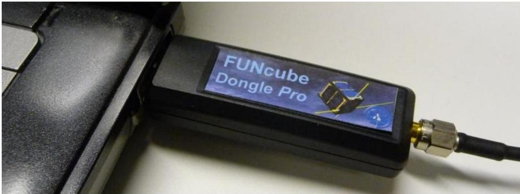
*Figure A.1 FUNcube Dongle Software Defined Radio*
