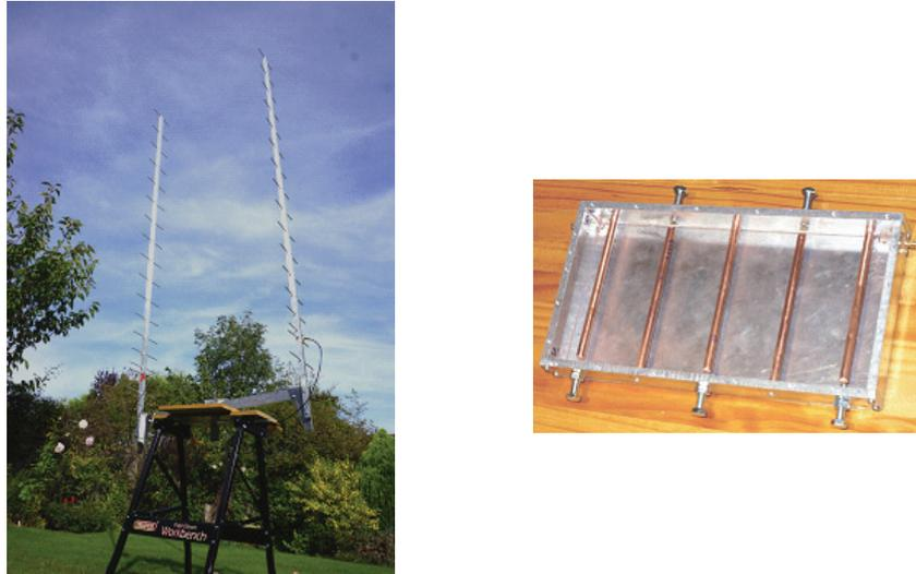
**Figure 2** Antenna and Interdigital Filter Detail
