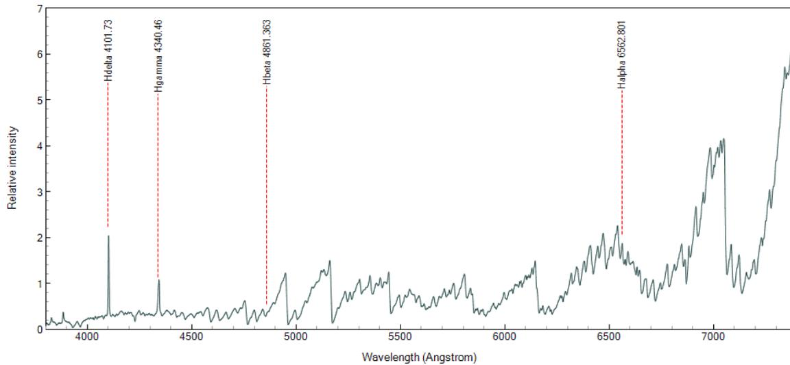
Spectrum of Mira taken by David Boyd on 2019 November 11. Total exposure of 120 sec with a LISA spectroscope on a C11 scope. The prominent hydrogen Balmer H-delta and H-gamma emission lines are generated by shock waves inside the atmosphere of pulsating red giants like Mira towards the maximum of their pulsation cycle. The rest of the spectrum is composed of saw-tooth-like features produced by absorption by TiO molecules in the cool atmosphere of the star.
