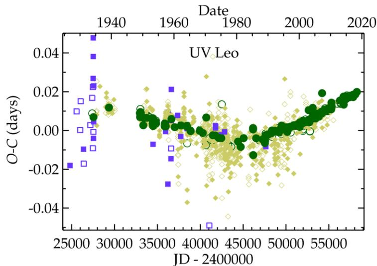
Figure 2: Historical O-C diagram of UV Leo showing the secular increase in period largely through one discrete period change around 1985. The low-amplitude cyclic variation can also be seen.
