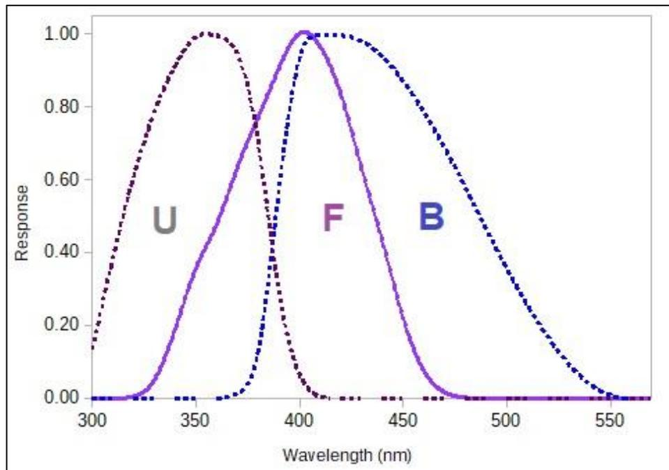
Figure 1: Normalised response of the new F band compared to Johnson U and B bands.
