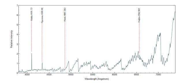
Spectrum of Mira taken by David Boyd on 2019 November 11. Total exposure of 120 sec with a LISA spectroscope on a C11 scope. The prominent hydrogen Balmer H-delta and H-gamma emission lines are generated by shock waves inside the atmosphere of pulsating red giants like Mira towards the maximum of their pulsation cycle. The rest of the spectrum is composed of saw-tooth-like features produced by absorption by TiO molecules in the cool atmosphere of the star.
