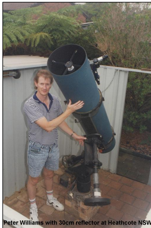
Figure 2: Peter Williams with his 30cm F6 Newtonian Reflector that was used for the bulk of his telescopic observations of variable stars and also for the discoveries of Comet C/1998P1 and V2576 Oph (photo taken in April 2006).
