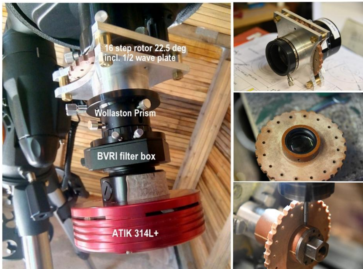
Figure 1. Dual Beam Polarimeter mounted on Celestron [C6], 150 mm objective Schmidt Cassegrain Telescope.
