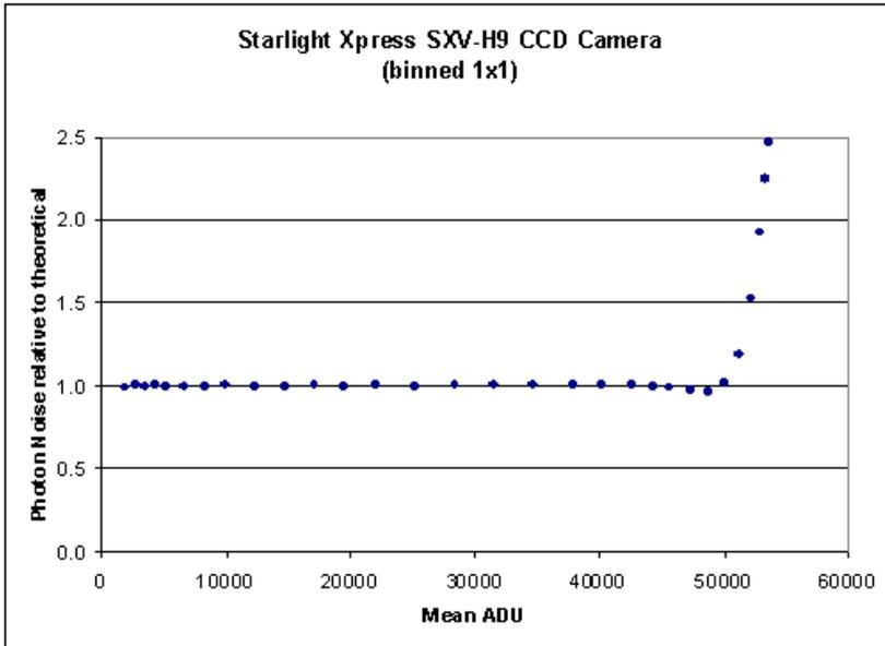
**Figure 4, Increase in Noise with ADU Counts per Pixel**
