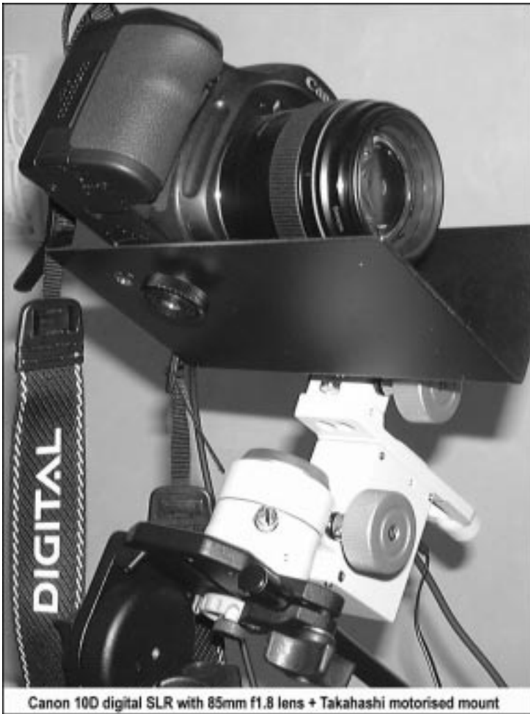
Fig 1: Canon 10D digital SLR with 85mm f1.8 lens on Takahashi motorised mount
