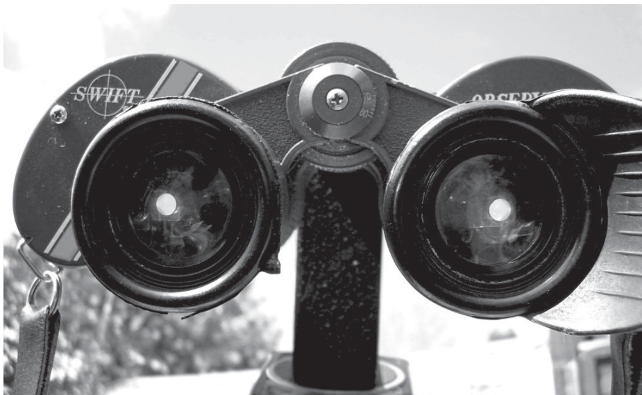
Figure 2: 16x70 with its exit pupil, side guard and clamp.
