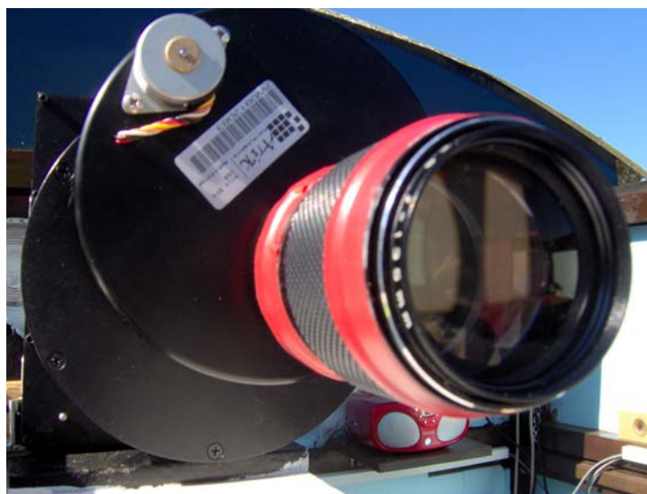
Figure 2: I used tape for masking parasite light.
