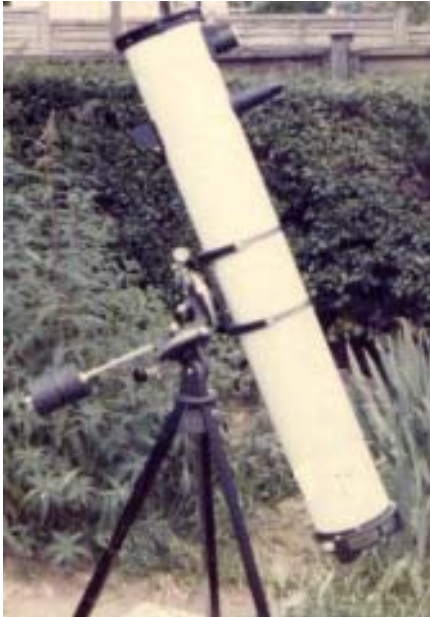
Figure 1: The 6inch F8 Newtonian which was used for the first Variable Star observations in 1975.
