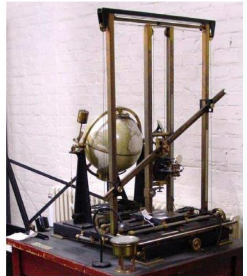
Figure 8. Wescott's metal Occultation Machine. (Courtesy the National Maritime Museum, Greenwich, London.)
