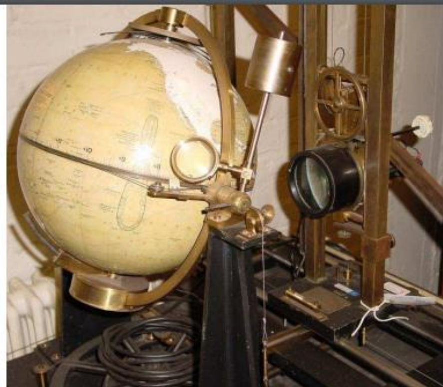
Figure 9. The Earth globe and Moon lens assembly. (Courtesy the National Maritime Museum, Greenwich, London.)
