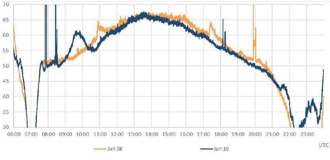
2021 Solar eclipse at 24 kHz from Basingstoke UK
