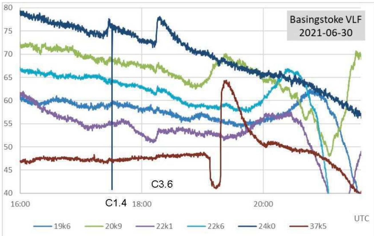
This recording by Paul Hyde shows activity on June 30<sup>th</sup>, both SIDs showing clearly at 24kHz. The other signals are far less clear, the flares occurring as they fade towards sunset. They do not show at all at 37.5kHz, with just a very odd transient visible around 19:00 – 19:30.
