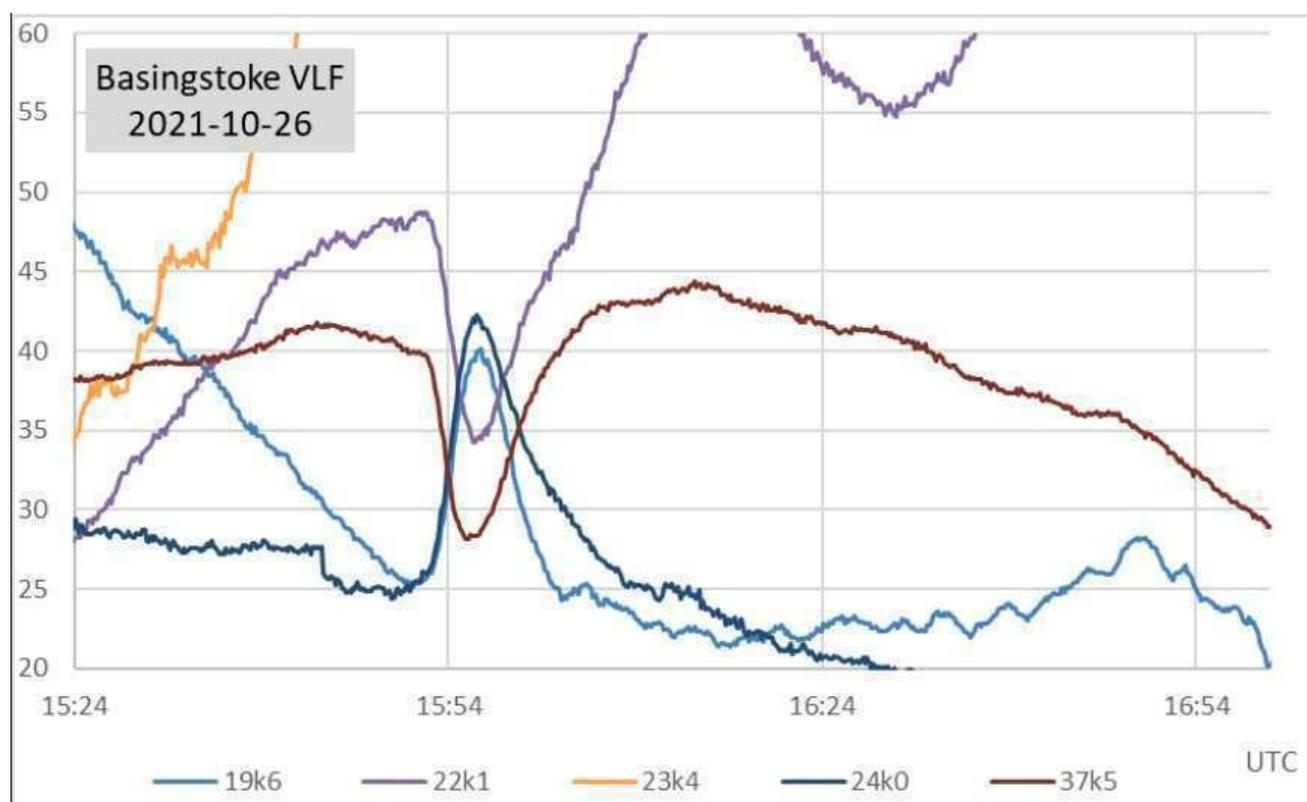
This recording from Paul Hyde shows the M1.0 flare peaking at 15:56UT on the 26<sup>th</sup>. The 23.4kHz signal is rising steeply into the sunset, but the other signals all show good clean SIDs.
