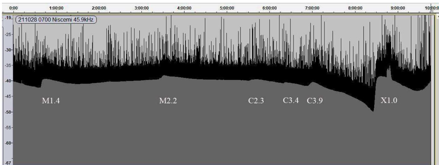
Colin Briden recorded the 45.9kHz signal from Niscemi, Italy, SIDs showing in the grey area, black indicating the raw signal data. Here all of the flares have produced ordinary 'shark fin' SIDs.
