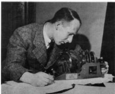
J. P. M. Prentice in 1934, using an aircraft navigating machine for converting RA and dec. into azimuth and altitude.
