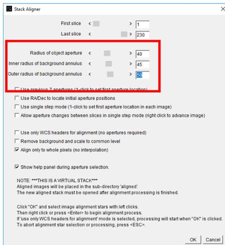
4. Select T1 and comp stars are standard and <Enter> to start alignment. When complete, aligned images are stored in **aligned** subfolder.
