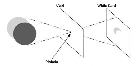
A simple pinhole projector made with two pieces of card.
