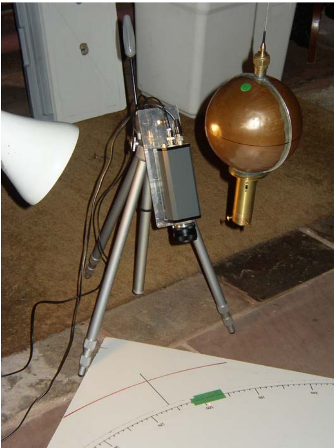
Figure 2. The original bob, laser, camera position and target scale. The anglepoise lamp on the upper left illuminates the area to optimise the image contrast between the target and the red laser trace. The target is green for the same reason. The copper ball-tap float pendulum bob still looks like what it was made from in this picture. The green sticker on the bob identifies the hemisphere.
