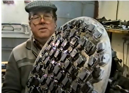
Jim Hysom in his workshop, holding the tool used for polishing large mirrors. (Taken from a 1991 video by Martin Moberley.)
