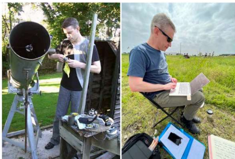
Left: Collimating the mirrors in Sir Patrick Moore's 12.5-inch Newtonian Reflector.
