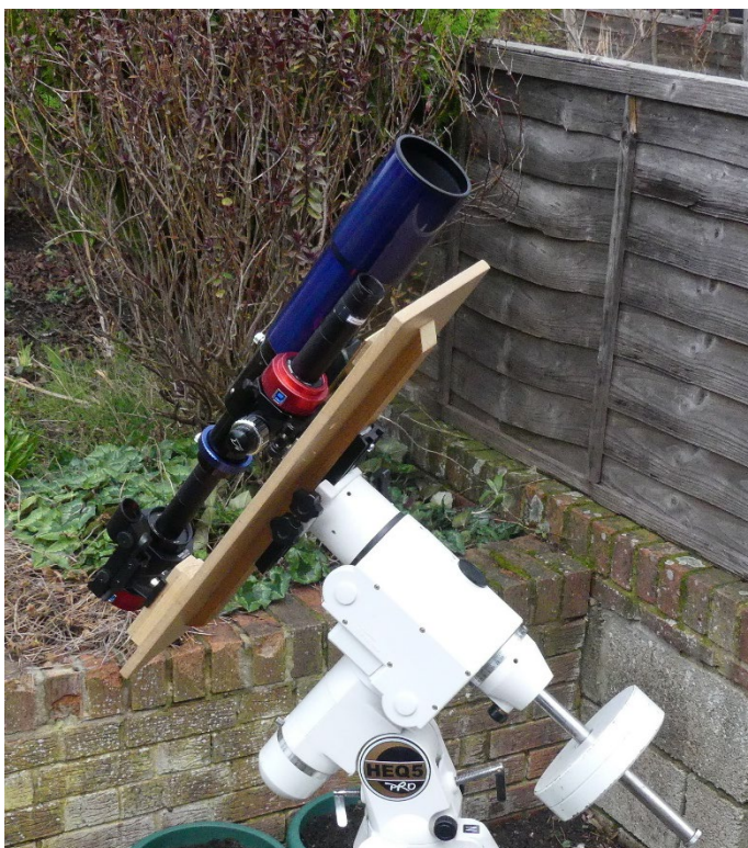
Figure 3. Complete setup for imaging Mercury's tail, including finder and guide camera.
