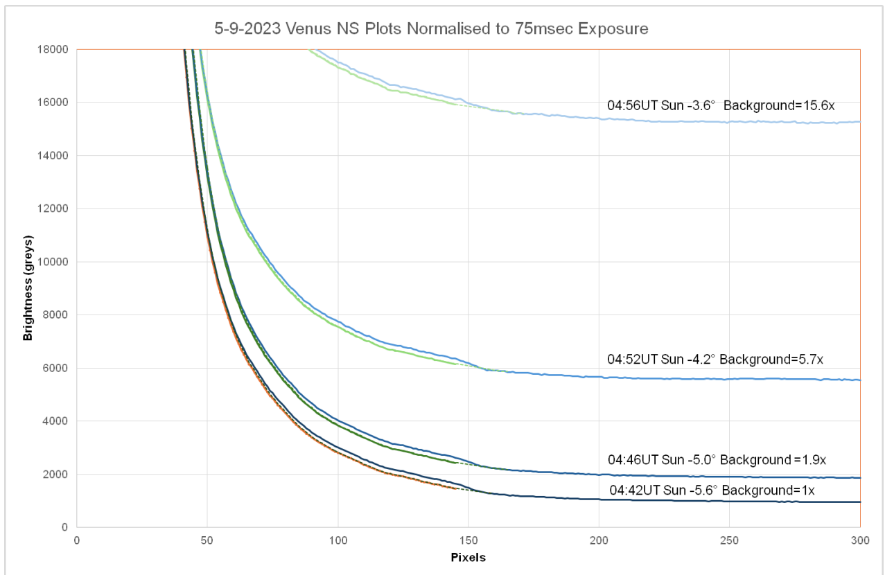
Figure 5: Line profile for images taken over a 14min. period on 5/9/2023 showing climbing sky brightness as the Sun approaches sunrise. Background brightness are given for each altitude relative to that at 04:42UT
