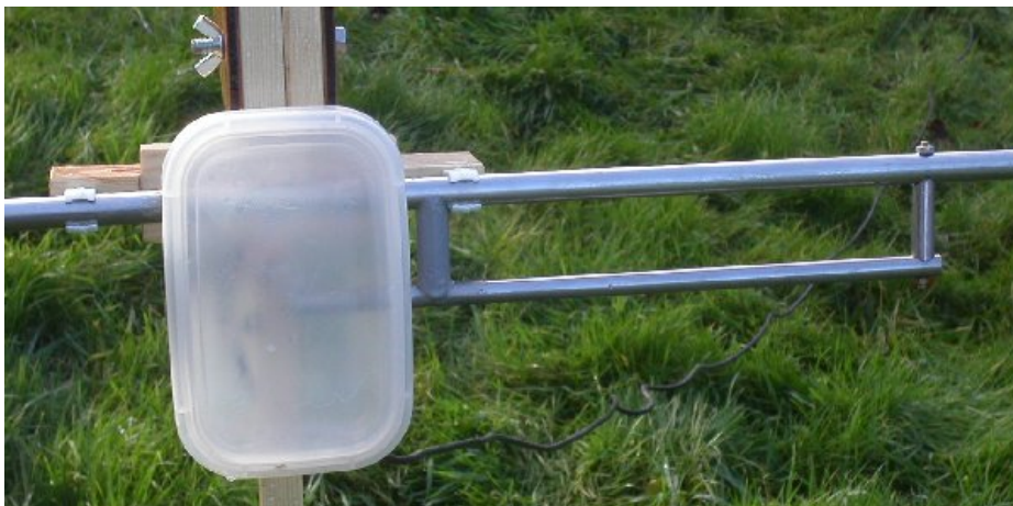
Figure 14 The finished driven element assembly
