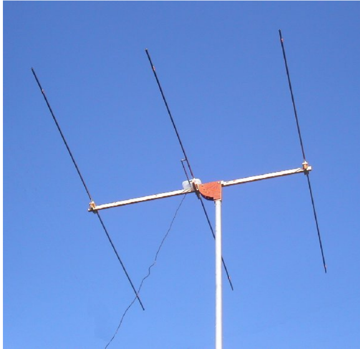
Figure 15 The completed Receive Antenna
