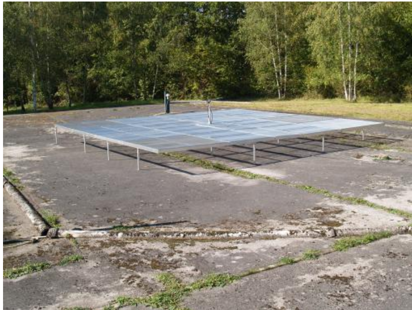
Figure 4 The BRAMS Tx antenna with improved ground plane
