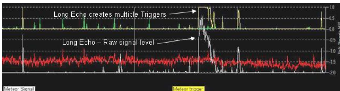
Figure 5 Example of Multiple Echo Triggers from a long Radar return (aircraft?)
