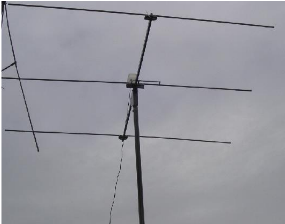
Figure 3.4 50MHz Yagi Antennas for Meteor Radar Reception
