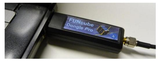
Figure A.1 FUNcube Dongle Software Defined Radio
