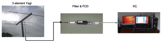
Figure 2.2 Graves Radar Receiver
