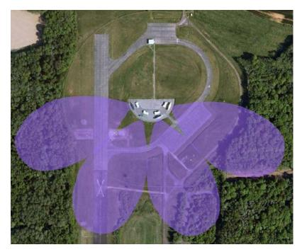
Figure 3.2 Southward Pointing Antenna beams
