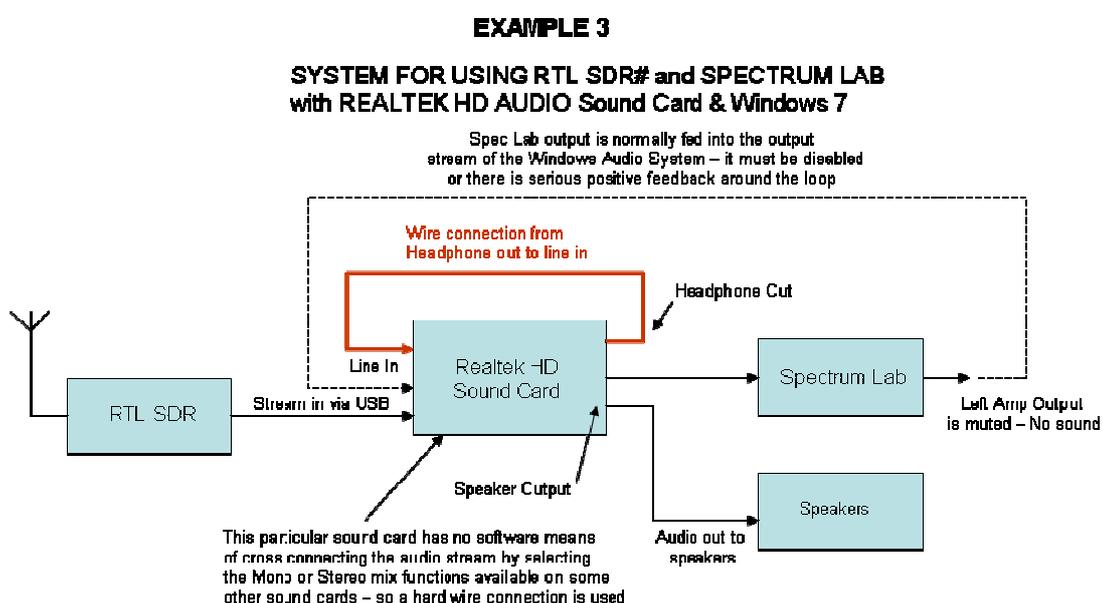
Figure 10 Hardware connection – Headphone to Line input
