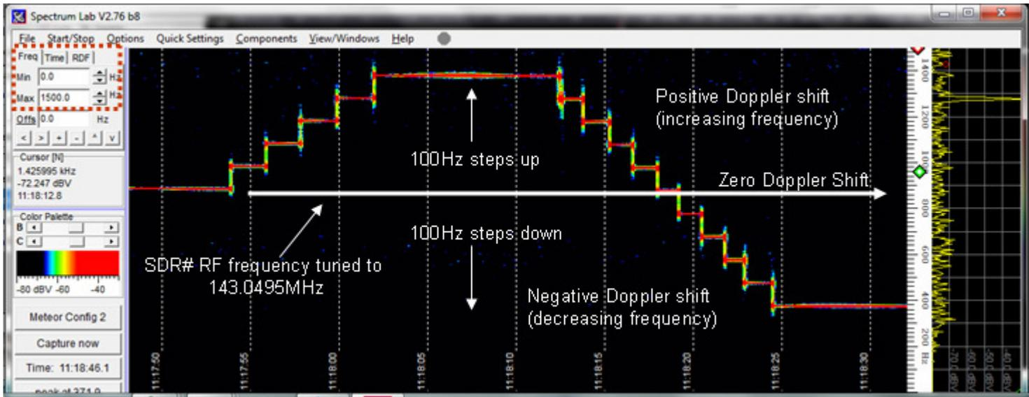
Figure 7 Spectrum Lab Waterfall Display – ‘Correct’ Doppler display
