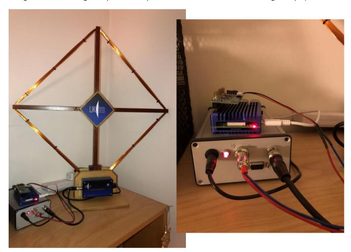
This then connects with the 2 pin header I put into input 1 of the AB Electronics ADC Pi HAT. The AB Electronics ADC Pi HAT pugs directly into the Raspberry Pi GPIO header.
