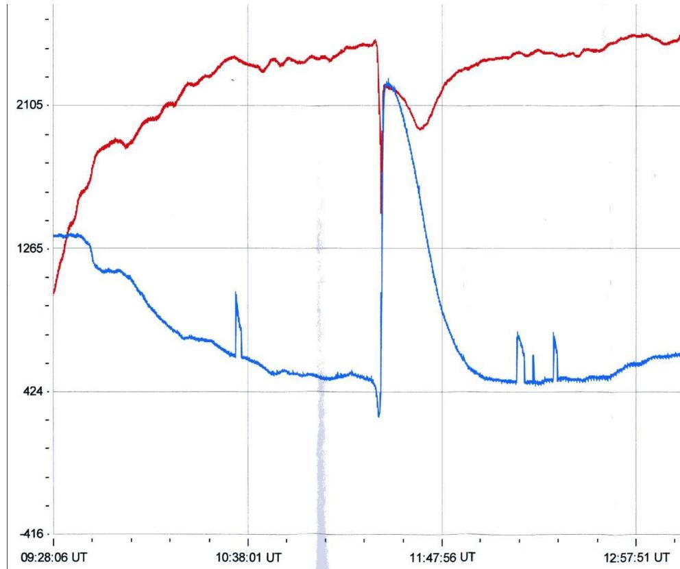
Red is 23.4kHz, blue is 37.5kHz. The response is good and exceeds that from Germany, thus proving my assumption wrong. The path to the north west should provide a little extra coverage before sunset.
