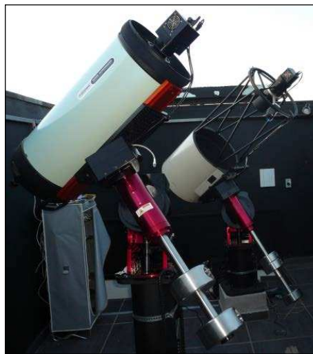
Figure 1. SONEAR 18: 457mm aperture f/2.9 telescope (Sandro Coletti mirror) with CCD camera at the primary focus, installed on a Paramount equatorial mount and remotely operated over the Internet. Cristóvão Jacques
