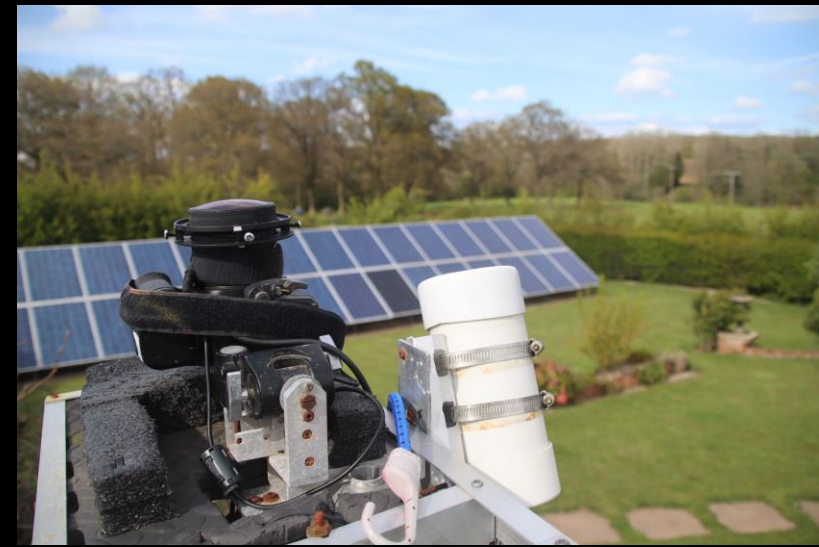
SQM (20 deg .fov), tilted 20 deg. N of Zenith, away from observatory panel lights with no direct or reflected view.
