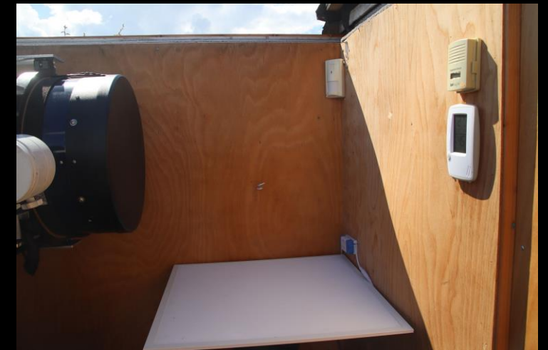
SQM (20 deg .fov), tilted 20 deg. N of Zenith, away from observatory panel lights with no direct or reflected view.
