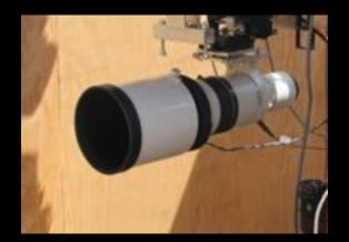
The 3° field of view 300 x2 mm fl 60Da camera system is typically picking up satellite crossings in most directions south of zenith an hour or so before dawn, of up to 3 per frame of a typical sequential 120 second exposures, increasing to about 20% of frames.
