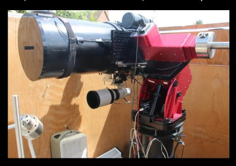
Piggyback on the RCOS, is a Canon D60a camera and 300mm FL x2 with 60Da camera.
