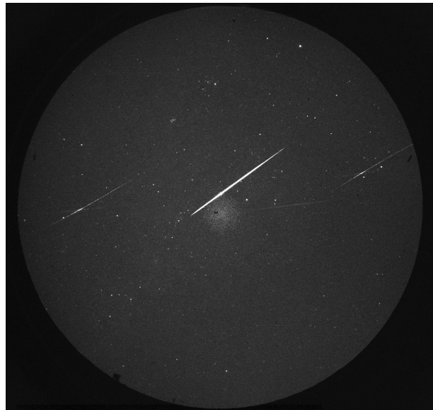
Figure 1: Na-rich meteor observed by the AMOS-Spec system on February 13, 2015. The meteor (0-order) is captured in the middle of the FOV along with the +1 and -1 order of its spectrum consisting solely of the Na I line.
