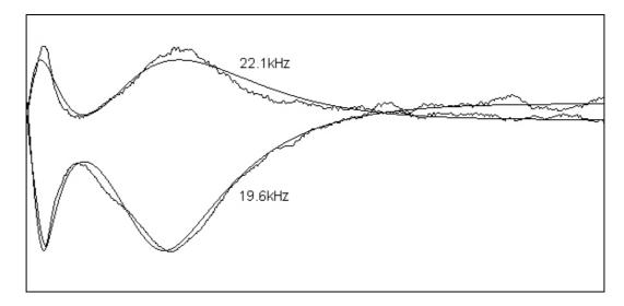
Where the smooth lines are the output of the model and the jagged lines are the observations.
