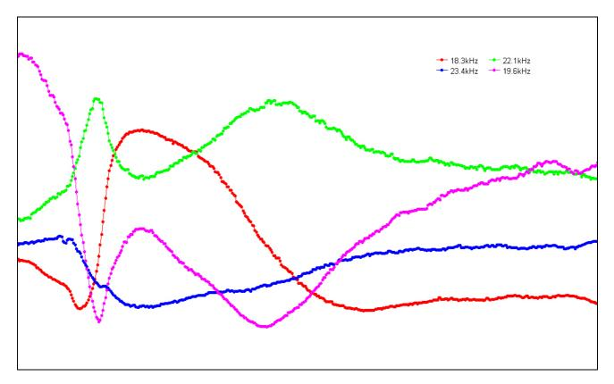
One thing is immediately obvious; the SID produced remarkably different effects at each of the four frequencies. Of particular note are the totally opposite effects at 19.6 and 22.1 kHz, which are also notable for having two prominent peaks (or troughs).
