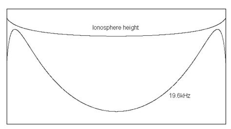
This shows the diurnal variation in the strength of the received signal as the height of the ionosphere drops from 78km during the morning to 71km at local noon and rises again to its original height during the afternoon.
