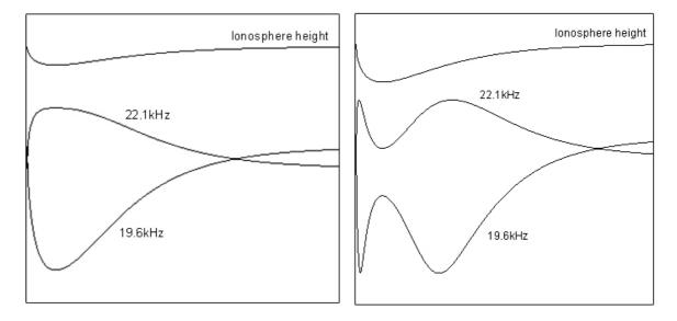
In the left-hand diagram the ionosphere starts at height just above 70km and drops by a small amount that takes it towards the height (69.2km) at which there is a maximum for 22.1kHz, but crucially not through it. This produces the characteristic single peak of a SID.
