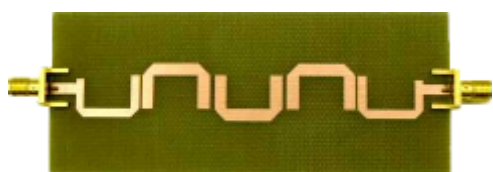
The 2.695GHz bandpass filter, bandwidth approximately 100MHz
