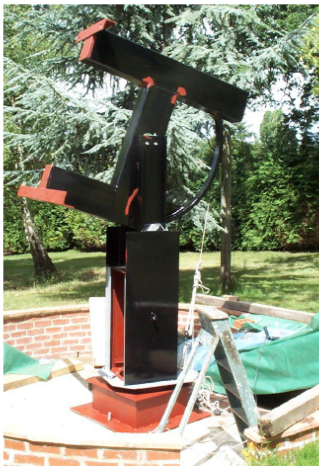
Final assembly of the Azimuth and Elevation mount. Last year's major project
