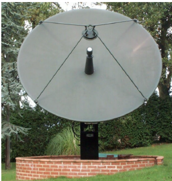
The telescope with its original Cassegrain feed suitable for frequencies of 10GHz and above
