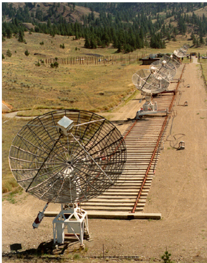
Figure 3: The 7-element Synthesis Radio Telescope at the Dominion Radio Astrophysical Observatory, near Penticton, British Columbia, Canada.
