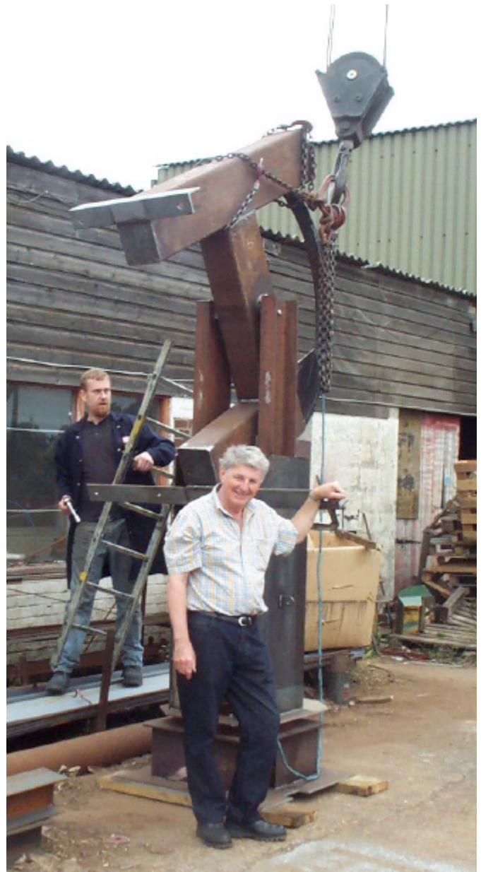
Ian Lever G8CPJ (front) attends a trial assembly of the elevation mount at the fabricators
